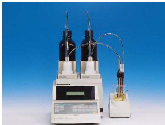
AT-500 Automatic Potentiometric Titrator with twin burettes mounted
